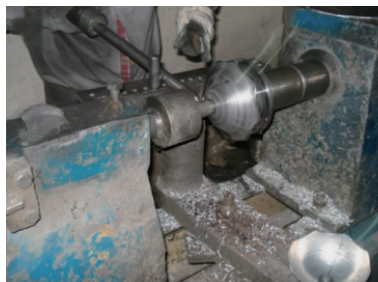
图5 八边形板坯旋压试验装配和成形过程 [16] Fig.5 Assembly diagram for octagonal blank spinning experiment and forming process [16]
