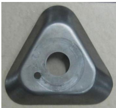
图4 去顶三角形锥台零件 [15] Fig.4 Triangular frustum parts with the top removed [15]
